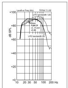
Figure 10. The free field frequency response of 7070A and 7071A subwoofers at different Bass Roll-Off settings.
